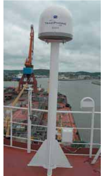
The antenna is 69.5 cm in height, 66.5 cm in diameter, and weighs 27 kg
